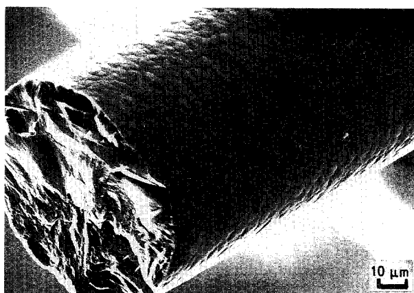
Figure 3 Scanning electron micrograph of as-received Sigma fibre.
